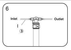
6.Connect the Drinking water Inlet hose(I) with lable ③ into the filter housing inlet. See Fig.6
