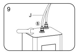
9.Connect the Boiling water outlet hose (J) with label ⑤ into the Tank outlet(Red Nut). See Fig.9
