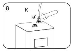
8. Connect the Drinking water Outlet hose(K) with label ④ into the Tank Inlet (Blue Nut). See Fig.8
