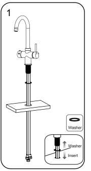
1.Insert the rubber washer (B) over the hoses into faucet shank, and mount the faucet on the basin. See Fig.1
