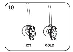
10. Tum on the water supply and check the water connections for leaks.
