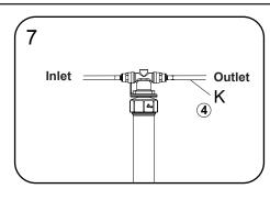
7. Connect the Drinking water Outlet hose(K) with label ④ into the filter housing outlet. See Fig.7
