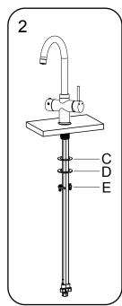
2.Slide the rubber gasket (C) firstly, metal washer (D) secondly, then the mounting nut (E) over the hoses onto the stem, and hand tighten them firmly. See Fig.2
