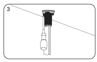
3. Use a Pgillips head screwdriver to thread the 2 screws. See Fig.3
